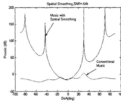
Fig. 3 Comparison of Conventional MUSIC with Spatial Smoothing technique in coherent multipath environment. Four coherent signals arrive at an 8-element linear uniform array at angles 30, -43, 70 and -81 degrees, respectively.
