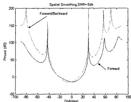
Fig. 4 Comparison of Forward Spatial Smoothing technique with Forward/Backward method. Five coherent signals arrive at a 9-element uniformly spaced array at angles -81, -43, 30, 57 and 70 degrees, respectively.
