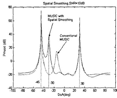
Fig. 1 Comparison of Conventional MUSIC with Spatial Smoothing technique for the case of two coherent waves and one incoherent wave received by an 8-element uniform linear array at angles 30, -30, and -45 degrees, respectively.
