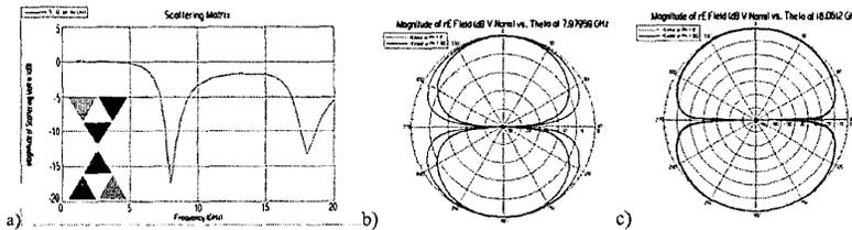
Figure 5. a) Antenna's  $S_{11}$  with one(x2) diagonal switch ON only. Antenna resonates at higher frequencies (8 GHz and 18 GHz) due to its reduced physical size. b,c) Radiation patterns at 8 GHz and 18 GHz.
