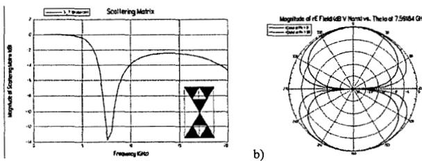
Figure 4(a,b). a)  $S_{11}$  of the antenna with all the switches connected (ON, state 111-111). The antenna functions at around 7.6GHz as expected. b) Radiation pattern at 7.6 GHz.
