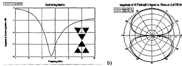
Figure 3(a,b). a)  $S_{11}$  of the antenna with all the switches disconnected (OFF, state 000-000). The antenna functions as a 13.8 GHz printed bowtie on a Silicon layer. b) Radiation pattern at around 13.8GHz.
