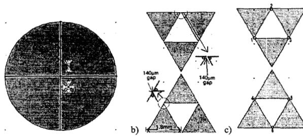
Figure 2(a,b). a) The antenna as etched on a quarter of a silicon wafer. Also shown below a design for circular polarization. b) The antenna's shape and dimensions. c) The switch positions and numbering
