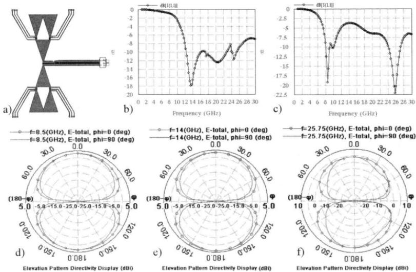
Figure 4. a) The proposed antenna design. b,c)  $S_{11}$  of the reconfigurable system for different states. d-f) Radiation patterns of the system for different switch states.
