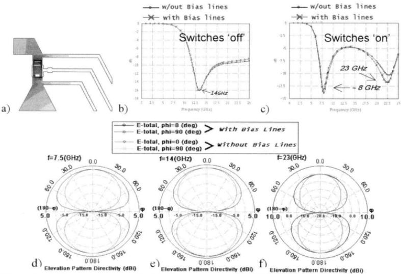
Figure 2. a) Current flow on the biasing network at 23GHz: black (high), gray (average), and white (minimum current flow). b,c)  $S_{11}$  of the system with and without bias lines for different states. d-f) Effect of the bias network on the radiation patterns.
