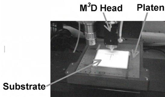
a) Figure 2. PIFA antenna during fabrication placed on the M<sup>3</sup>D platen. The M<sup>3</sup>D still head can be seen.
