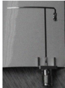
b) Figure 3. The fabricated PIFA antenna on photographic paper substrate.
