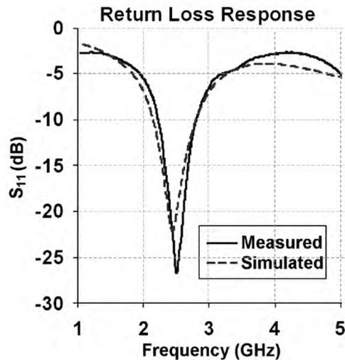
Fig. 4. The simulated and measured return loss response of the PIFA on paper (superimposed).
