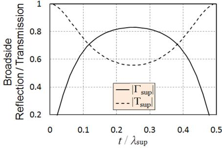
Fig. 2. Magnitudes of the broadside reflection and transmission coefficients versus the electrical thickness of a planar dielectric layer of  $\epsilon_r=10.8$  embedded in free space. An incident plane wave is assumed.
