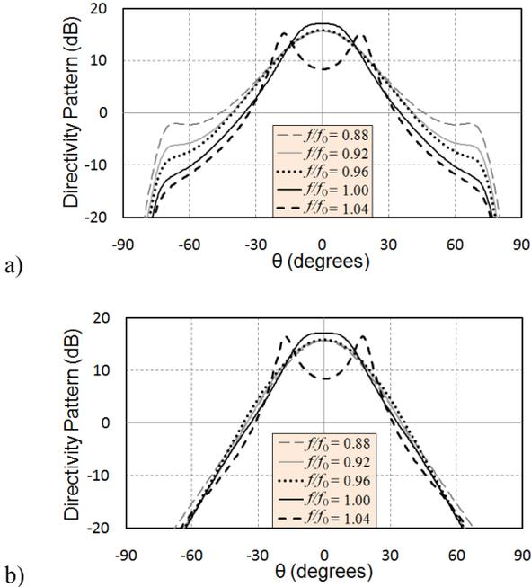
Fig. 8. Theoretical (a) E- and (b) H-plane directivity patterns at specific frequency points for the CRA in Fig. 6 using  $\epsilon_r=10.8$ ,  $h=\lambda_0(f=f_0)/2$ ,  $t_1=\lambda_{sup}(f=f_0)/4$ ,  $t_2=0.8h$ ,  $t_3=2t_1$ , and  $\lambda_0(f=f_0)/20$  feed-PEC spacing.
