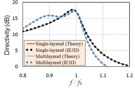
Fig. 9. Broadside directivity versus frequency curves of the single-layered and multilayered CRAs in Fig. 1 and 6, respectively.
