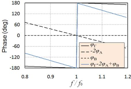
Fig. 3. Broadside variations with frequency of the phase shifts illustrated in Fig. 1(b) and evaluated in (1).  $\epsilon_r=10.8$ ,  $h=\lambda_0(f=f_0)/2$ , and  $t=\lambda_{sup}(f=f_0)/4$ .
