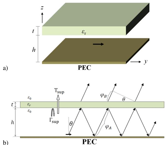
Fig. 1. (a) A single superstrate layer CRA, and (b) ray-tracing method for radiation analysis. A horizontal infinitesimal dipole feed is assumed.
