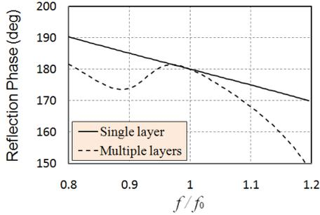
Fig. 7. Broadside reflection phase versus frequency curves of the single and multilayered superstrates in Fig. 1 and 6, respectively.
