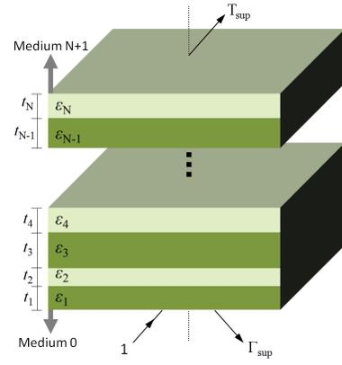
Fig. 5.  $N$ -layers of infinite, planar, and lossless stacked dielectrics.
