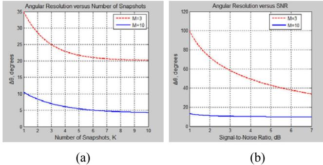
Figure 2. Resolution (a) versus the number of snapshots for SNR= 6 dB and (b) versus SNR for K=1.
