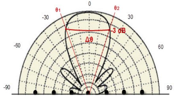
Figure 1. The ULA configuration and definition of its broadside resolution,  $\Delta\theta$ .
