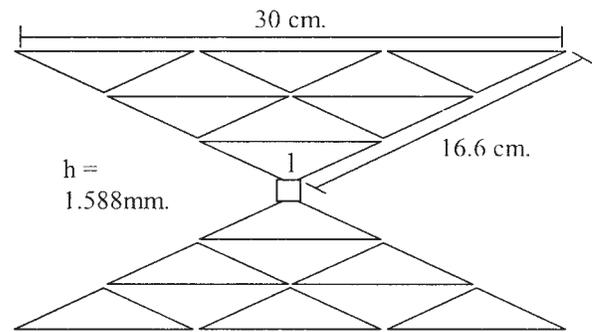
Figure 1 Reconfigurable antenna structure
