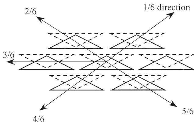
Figure 3 Order in which the elements are chosen to create the input data for the neural network
