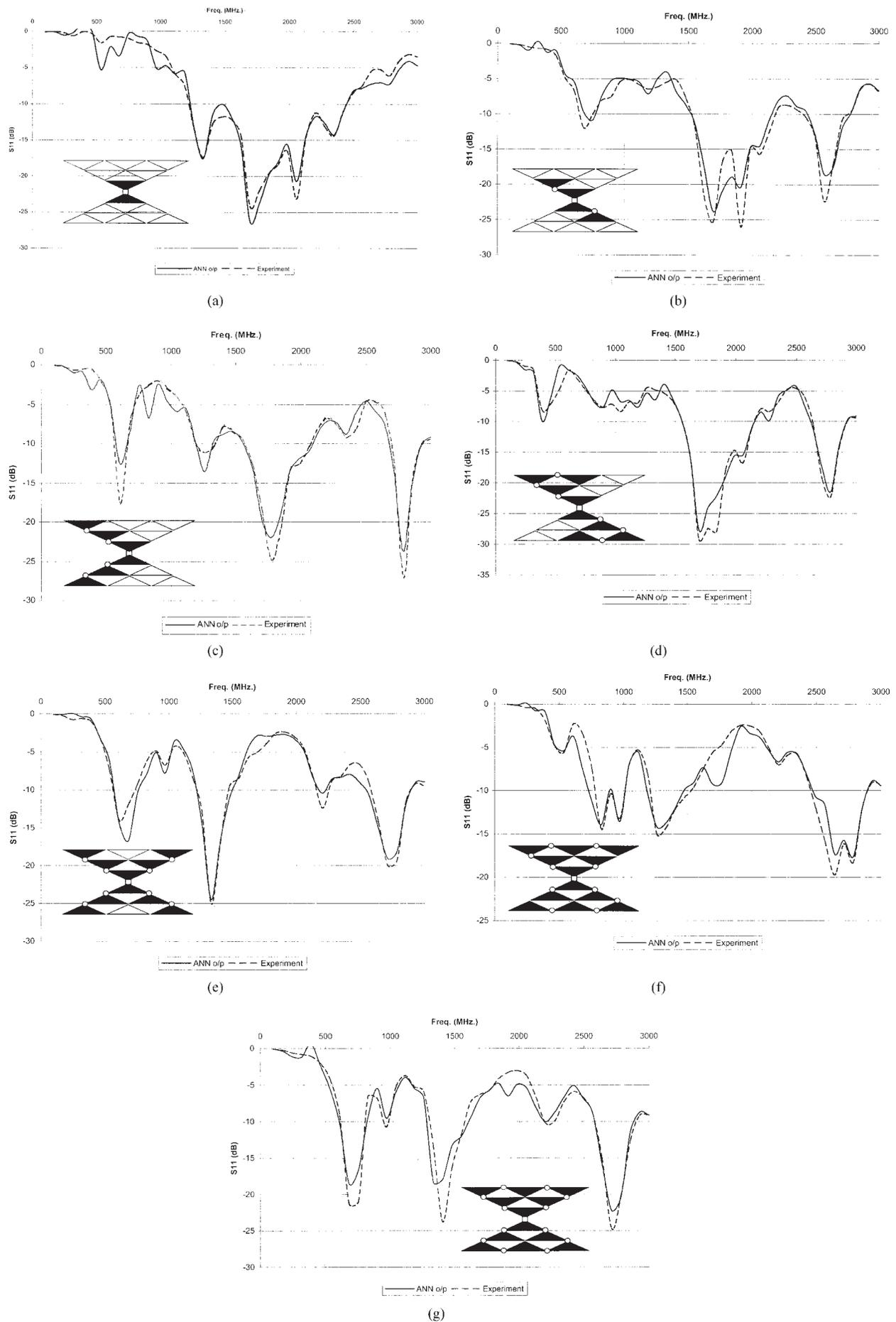
**Figure 4** (a)–(g) Plots showing the neural network output as compared to the experimental results (the ON switch positions on the antenna structure are marked with small open circles and the corresponding activated array elements are marked with small filled triangles)
