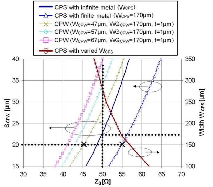
Fig. 3. CPS and CPW line characteristic impedance as it varies with the slot width ( $S_{\text{CPW}}$  or  $S_{\text{CPS}}$ ) and the width of the metal conductor ( $W_{\text{CPS}}$  for the CPS line). A 20- $\mu\text{m}$  slot was used in the CPS line plot.
