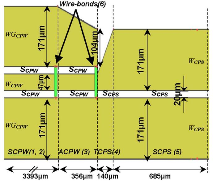
Fig. 4. Final CPW–CPS transition with dimensions and names of the different transmission line sections as defined in Fig. 1. The total length of the back-to-back configuration was  $2 \cdot 4300 = 8600 \mu\text{m}$ .
