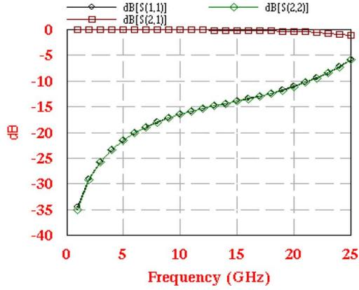
Fig. 2. Simulated  $S$ -parameters of the back-to-back initial transition with 600- $\mu\text{m}$ -long lines showed very good response up to 20 GHz. A gradual performance decline at higher frequencies can be noticed.
