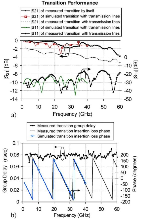
Fig. 5. Measured and simulated back-to-back transition performance. (a) Magnitude of insertion loss and reflection coefficient. (b) Group delay and insertion phase of  $S_{21}$  for the transition with all transmission lines attached.
