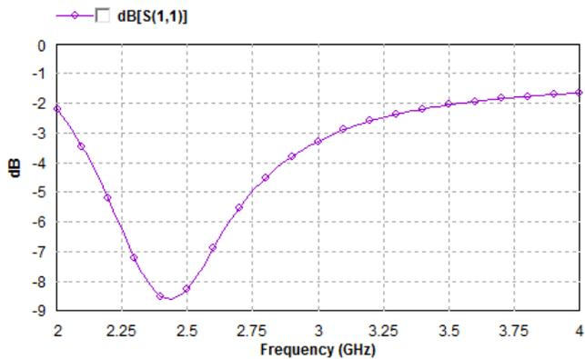
Fig. 2. Simulated |S<sub>11</sub>| characteristics of the QR Code Antenna.
