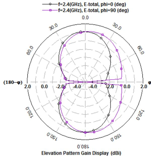
Fig. 5. Radiation pattern of the QR code antenna at the resonant frequency (2.4 GHz) in the two principal planes of the printed structure.
