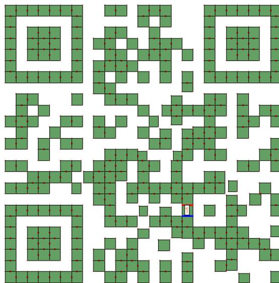
Fig. 1: Simulated model of the [www.sdsmt.edu](http://www.sdsmt.edu) QR code antenna, illustrating the device structure and the feeding port.
