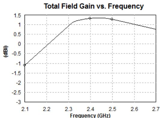
Fig. 4. Gain of the QR Code Antenna.
