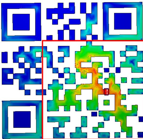
Fig. 3. Current density distribution on the QR code antenna. The red rectangle illustrates the predominantly active area of the antenna where a continuous conducting path exists.
