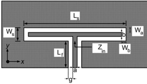
Fig. 1. Schematic of the CPW-fed single folded slot antenna. The shadowed (gray) areas represent metal areas.
