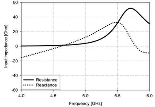
Fig. 3. Simulated input impedance of the modified folded slot antenna design after changing the dimension  $W_a$ . The input resistance is  $50 \Omega$  at 5.775 GHz. The reactance is zero at the same frequency.
