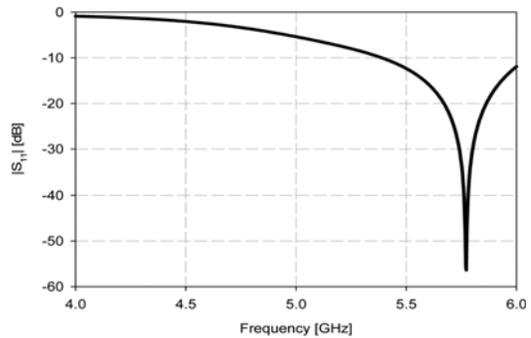
Fig. 4. Simulated return loss of the folded slot antenna with the dimensions shown in Table I(b). The CPW line's effect is considered in these results.
