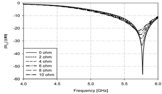
Fig. 7. Simulated return loss of the presented design at 5.775 GHz for different forward resistance values of the p-i-n diodes. The resistance deteriorates the return loss and slightly shifts the resonant frequency.
