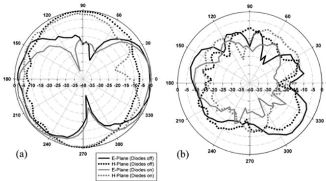
Fig. 12. Measured normalized E- and H-plane radiation pattern at 5.25 (diodes OFF) and 5.775 GHz (diodes ON): (a) co-pol radiation patterns, and (b) cross-pol radiation patterns.
