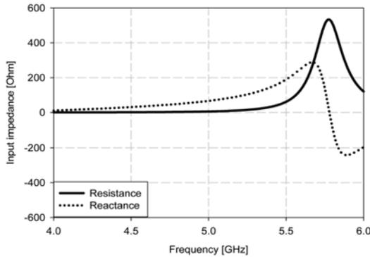
Fig. 2. Simulated input impedance of the initial folded slot antenna design. The resonance occurs at 5.775 GHz.
