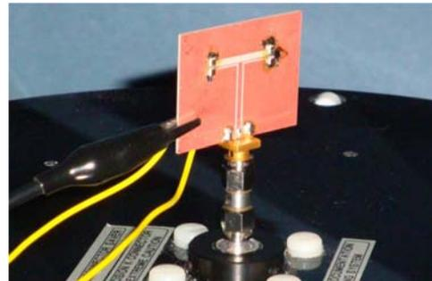
Fig. 9. The fabricated antenna during measurements. The diodes are biased from the back side of the substrate through vias (made only for illustration purposes). The dc ground is connected to the CPW ground.
