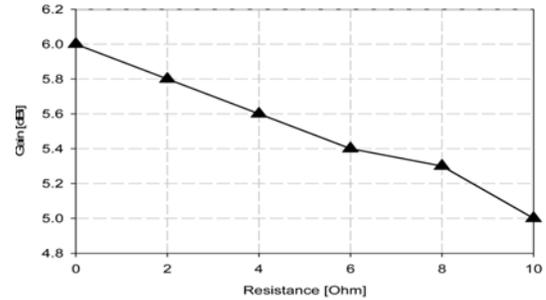
Fig. 8. Simulated gain response of the presented design with respect to different values of the forward bias resistance at 5.775 GHz. The gain deteriorates as resistance values increase.
