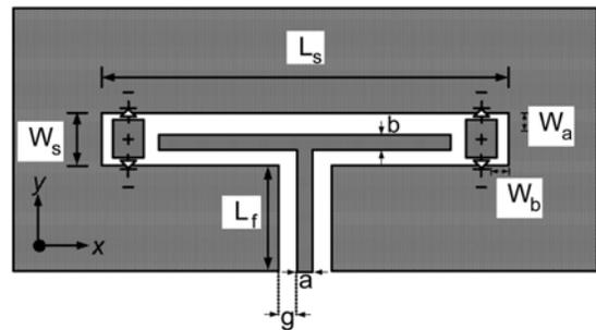
Fig. 5. Schematic of the reconfigurable folded slot antenna. The connection between the metallic strip and the ground plane is controlled by the diode's state. The dimensions are as in Table I(b), except for  $L_s$ , which is 21.22 mm.
