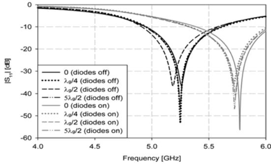
Fig. 6. Return loss of the reconfigurable antenna at both bands for various dc bias lines. The length of the bias lines, with respect to the guided wavelength at 5.25 GHz, practically does not affect the resonant frequency of the antenna at both bands.
