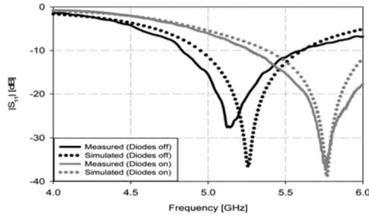
Fig. 10. Measured and simulated return loss response of the reconfigurable folded slot antenna. Measured results are very close to simulated ones. The effect of the dc bias cables is negligible.
