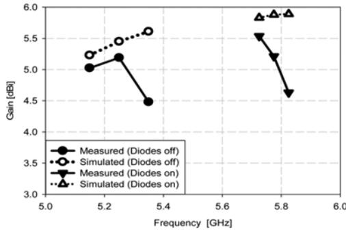
Fig. 11. Measured and simulated maximum gain of the reconfigurable folded slot antenna. The gain response does not change with the reconfigurability, and it exhibits similar values in both bands.
