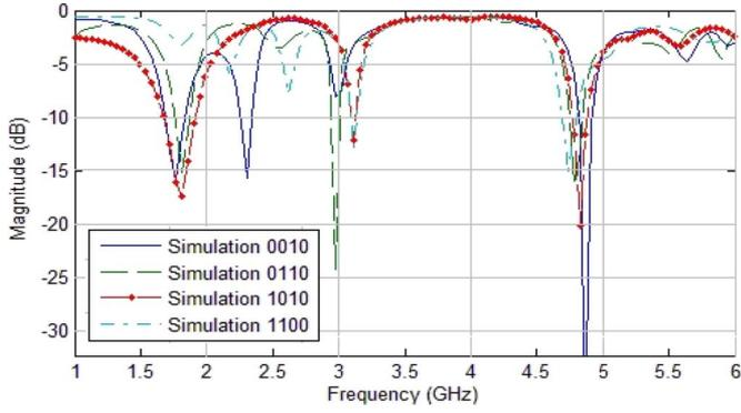
Fig. 3. Antenna resonances for different diode states: 0—OFF, 1—ON.
