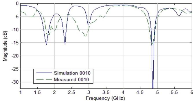
Fig. 8. Measured and simulated  $|S_{11}|$  comparison for the 0010 antenna state.
