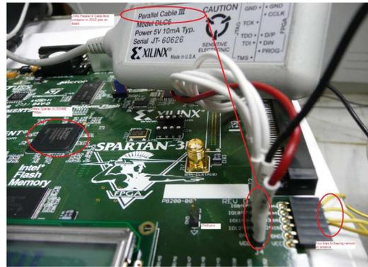
Fig. 7. The parallel III cable with FPGA board.
