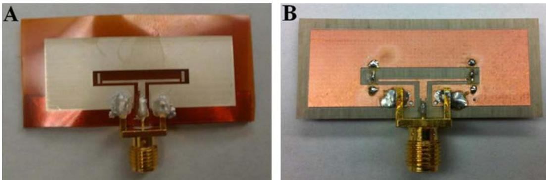
FIG. 3. (a) The direct-write printed CFSA and flexible folded-slot dipole antenna on Kapton<sup>®</sup> substrate. (b) Reference antenna made of copper.
