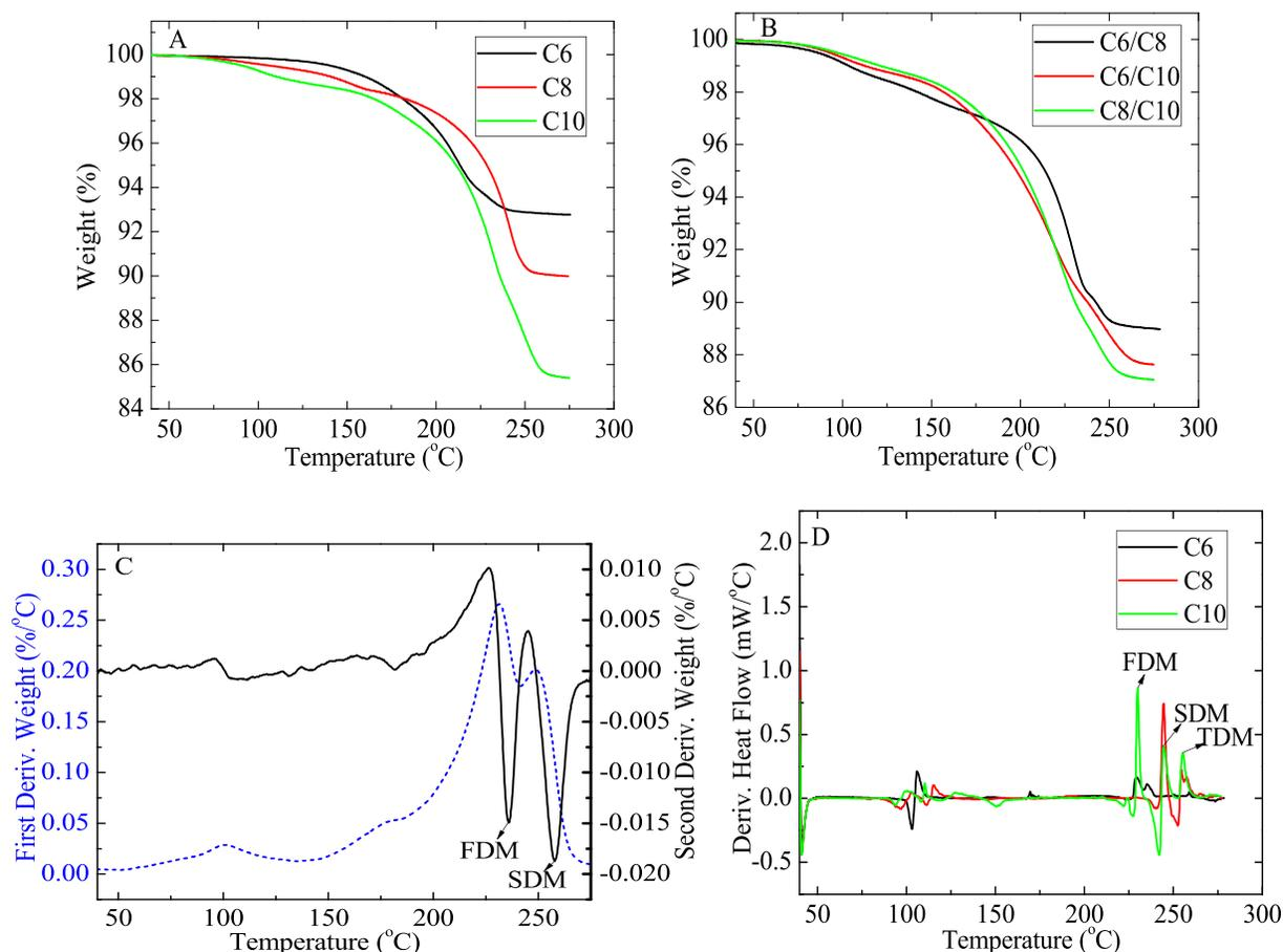
FIG. 1. (a) TGA curves for C6, C8, and C10 particles. (b) TGA curves for C6/C8, C6/C10, and C8/C10 particles. (c) First derivative and second derivative TGA curves for C10 particles. (d) First derivative DSC curves of C6, C8, and C10 particles.
