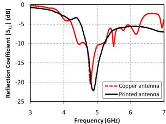
FIG. 4. The input reflection coefficient of the printed antenna compared to the reference antenna.
