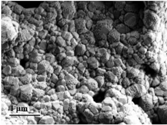
FIG. 2. SEM image of sintered pattern at 240 °C for an hour.
