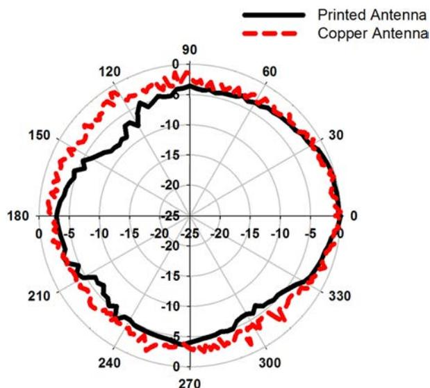
FIG. 5. Normalized radiation pattern of the printed CFSA and of the reference copper antenna in the principal radiation plane illustrating omnidirectionality and the suitability of the nanoinks for flexible antenna development.
